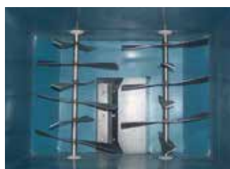
Dual Agitators Designed for Constant Flow
