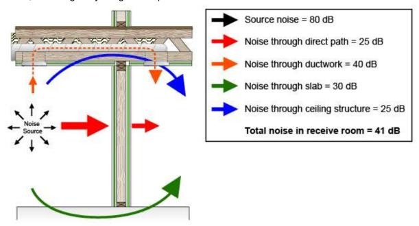
This diagram illustrates some simple flanking noise paths. The yellow arrow is direct sound - what you would measure in a lab to arrive at an STC rating, etc. - the red and blue paths are some simple "flanking paths". Often, these paths are more important than the direct, yellow, path at many frequencies.
