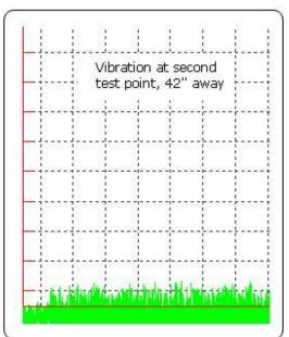
The test specimen was 2 layers of 5/8" drywall damped with Green Glue. This audio file demonstrates the dramatic noise decay over 8 feet in a Green Glue damped 5/8" drywall panel. The majority of noise in the second segment is simple background noise.
